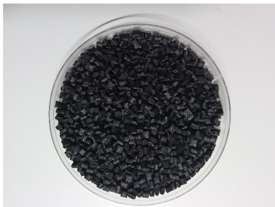
REAMIDE® Recycled Nylon Resin Made from Intake Manifolds
